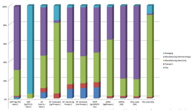
The evaluation of the Life Cycle Assessment results of the roofing tiles shows that the environmental impacts in all environmental categories are dominated by energy consumption during the manufacturing process (electricity and thermal energy from natural gas) in the factory.
